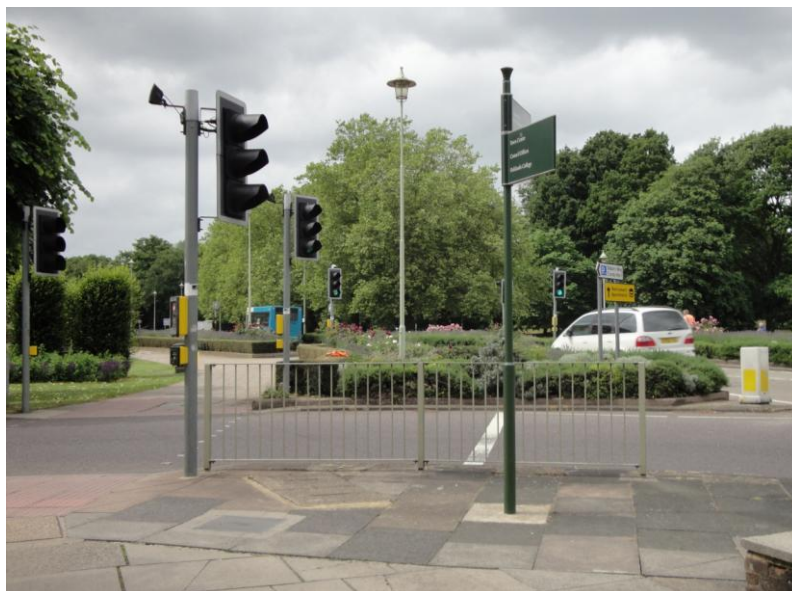
Fig 22 - Where new pedestrian guard rail has been introduced it is of a standard type but key to its integration in the street scene is the fact that it has been painted in BS12B21
